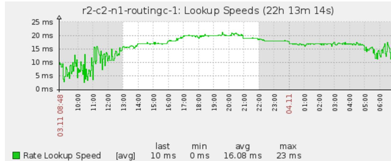
By enabling async operations inside of opensips, this all changed. Routing speeds matched synthetic benchmarks and temporary spikes in lookup speeds caused by changes in the rate structure were buffered by the asynchronous db connections.
